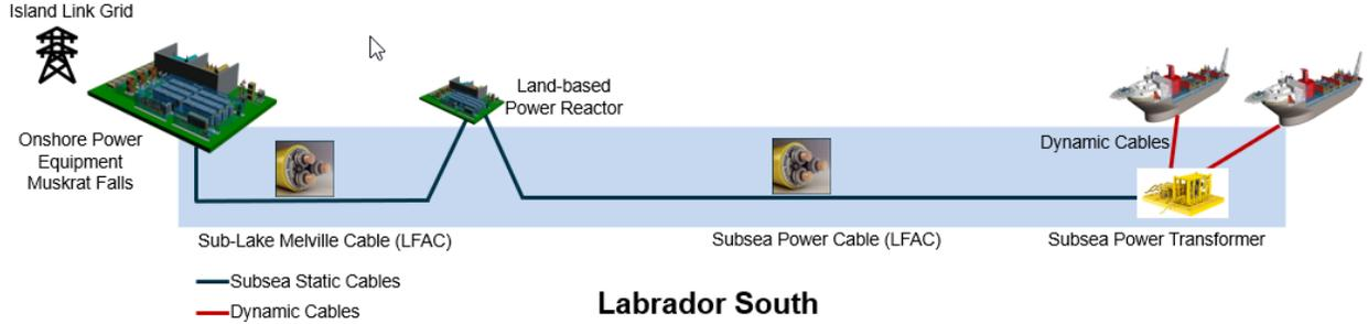
**Figure 8-7: Sample Layout 2x45MW FPSO Labrador South**
