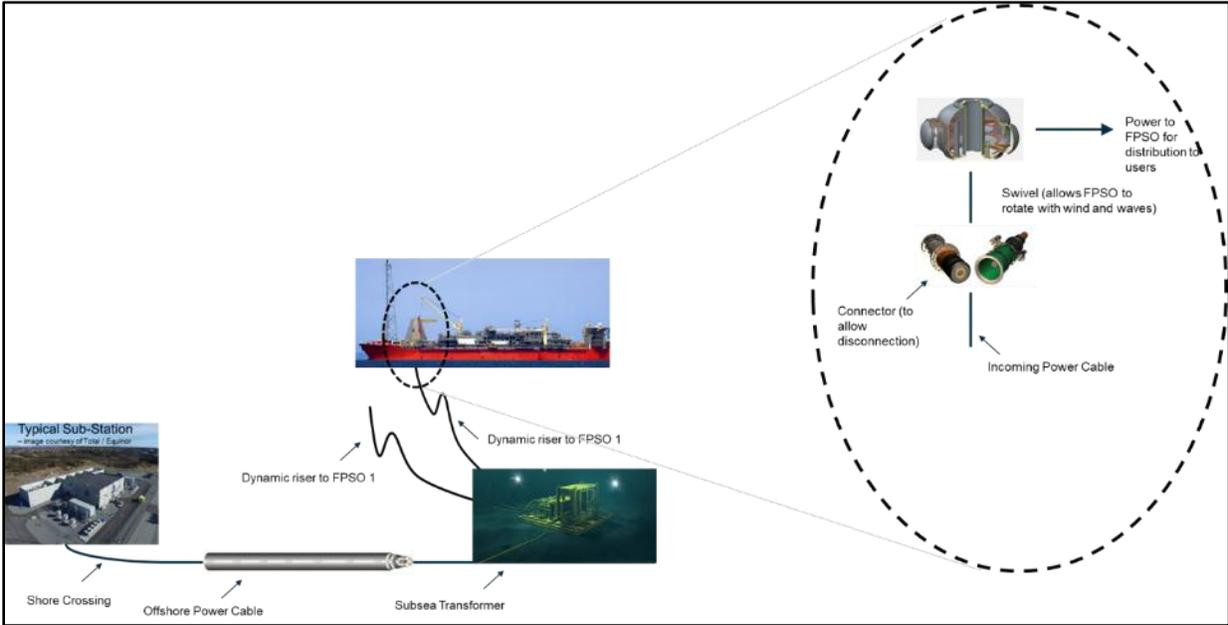
Figure 7-2: Low Frequency AC Power Supply to Ship Shaped FPSO
