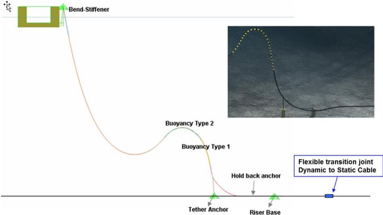
**Figure 8-18: Typical dynamic subsea cable or umbilical riser configuration**
