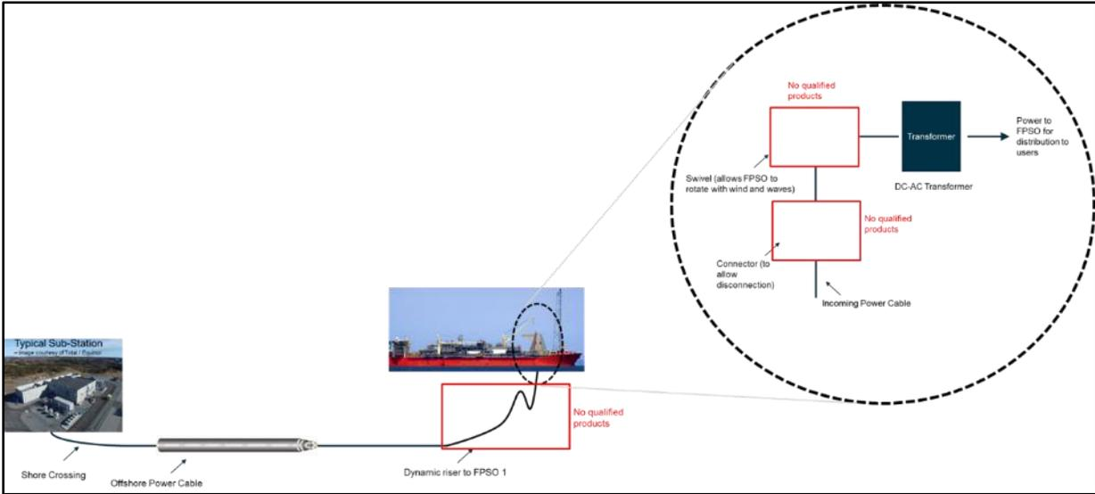
Figure 7-1: HVDC Power Supply to Ship Shaped FPSO
