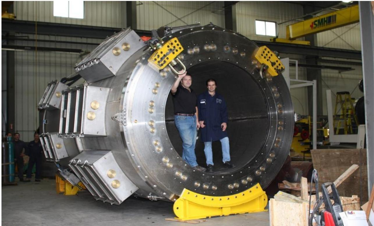
Figure 8-28: OSX-3 MVES, Exp, IP66, 18 x 11kV @ 650A plus 6 x 6.6kV @ 600A, approximately 5m tall - Focal
