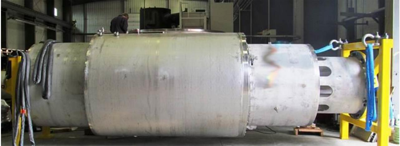
**Figure -: BZ-25 MVES – Ex o, IP66, 9 x 35kV @ 400A sliprings, approximately 8.5m tall – Focal**
