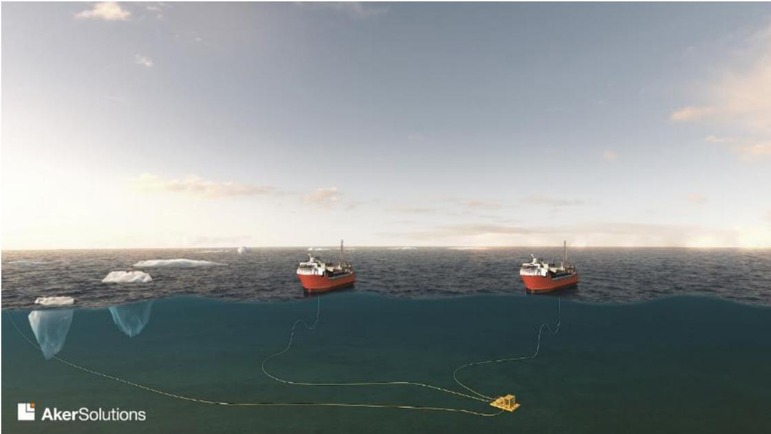
**Figure 1-1 Power from shore utilizing a subsea transformer for voltage stepdown and power distribution**
