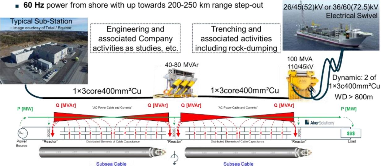
**Figure 8-4: Example AC transmission with reactive compensation in the middle of the cable run (Aker Solutions)**
